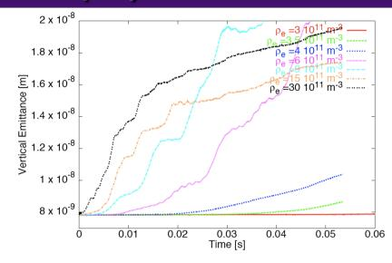
Figure 7.8. Vertical emittance as a function of time for different values of electron cloud density, and Q'=2 (for LHC at injection).
