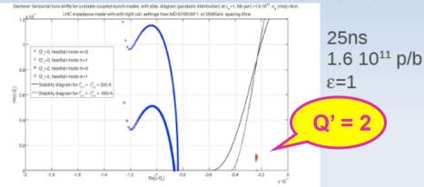
Points in blue are "rigidbunch" modes → can be damped by feedback.
