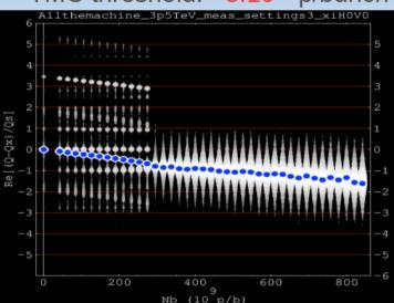
Coupled-bunch modes (each point = one possible coupled-bunch mode along the train, unstable if above the octupoles stability diagram)
