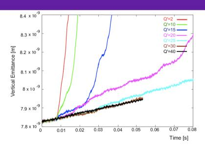
Figure 7.11. Vertical emittance growth for different chromaticities, for LHC at injection,  $\rho_e=6\times10^{11}~{\rm m}^{-3}$
