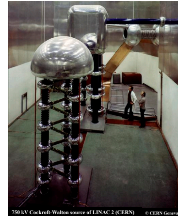
750 kV Cockcroft-Walton source of LINAC 2 (CERN) © CERN Geneva
