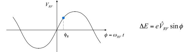
The phase of the synchronous particle is now  $\phi_s > 0$  (circular machines convention)
