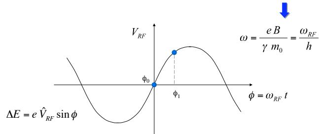
In order to keep the **resonant condition**, the particle must keep a **constant energy**.
