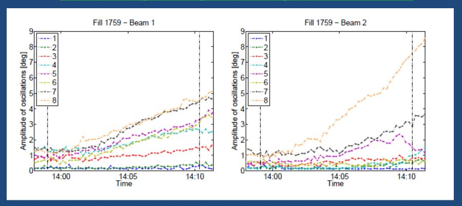
Amplitude of phase oscillations during acceleration cycle for 8 bunches (with different longitudinal emittances) of Beam1 (left) and Beam2 (right). Dashed vertical lines indicate start and end of the ramp.
