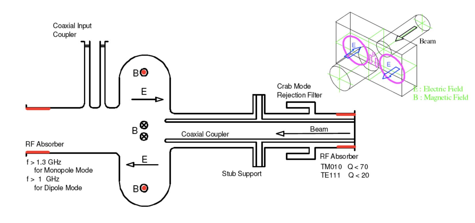
Figure 3: Conceptual design of the KEKB crab cavity (Top view) and schematic drawing of squashed cell shape cavity is shown upper right.
