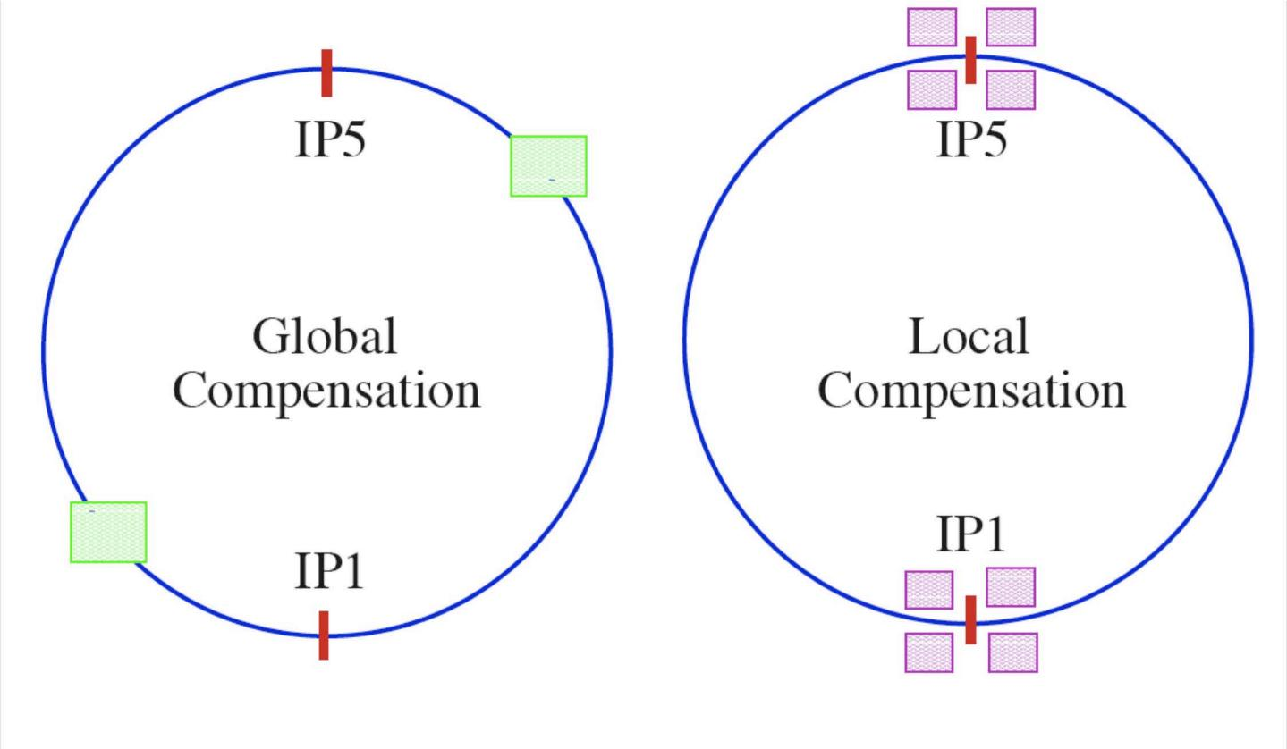
Figure 3: Schematic of global and local crab compensation at two IPs for LHC upgrade.
