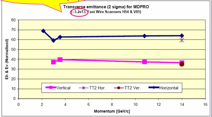
$\Rightarrow \boldsymbol{\varepsilon}_x (1\sigma, \text{norm}) \approx 16 \ \mu\text{m} \text{ and } \boldsymbol{\varepsilon}_y (1\sigma, \text{norm}) \approx 9 \ \mu\text{m} \text{ before CT}$
