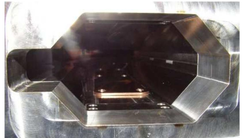
The electrode impedance consists of two contributions: a resistive wall impedance due to a finite conductivity of the electrode and a strip-line impedance since the stripline is created between the electrode and the vacuum chamber wall.
