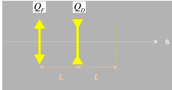
5) Derive the transfer matrix of a symmetric FODO cell (see Figure below) in the thin-lens approximation in which the drift spaces are replaced by dipole magnets of length  $L$  and bending radius  $\rho_0$ , to recover the result of page 47. Using the definition of the dispersion function, deduce the dispersion functions at the location of the focusing quadrupole  $Q_F$  and at the defocusing quadrupole  $Q_D$ . Perform the numerical applications for the following case:
