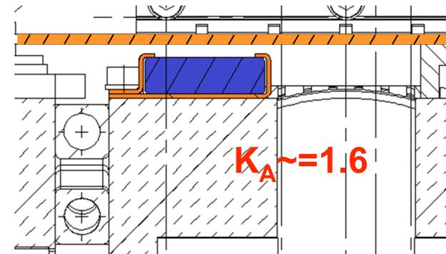
$K_A$  = Surface of the sink / surface of the ferrite
