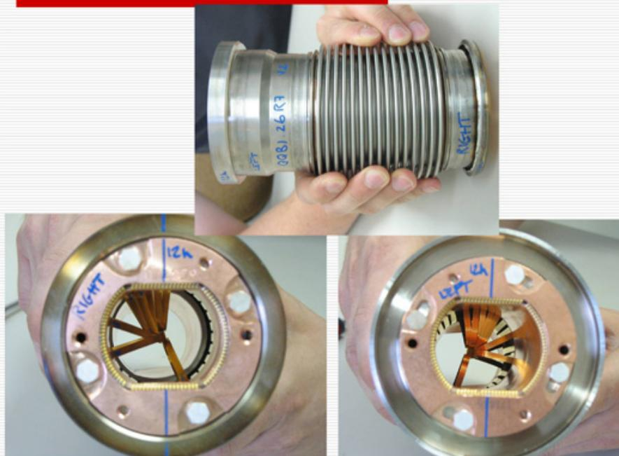
QQBI.26R7 V1 bending angles out of tolerance
