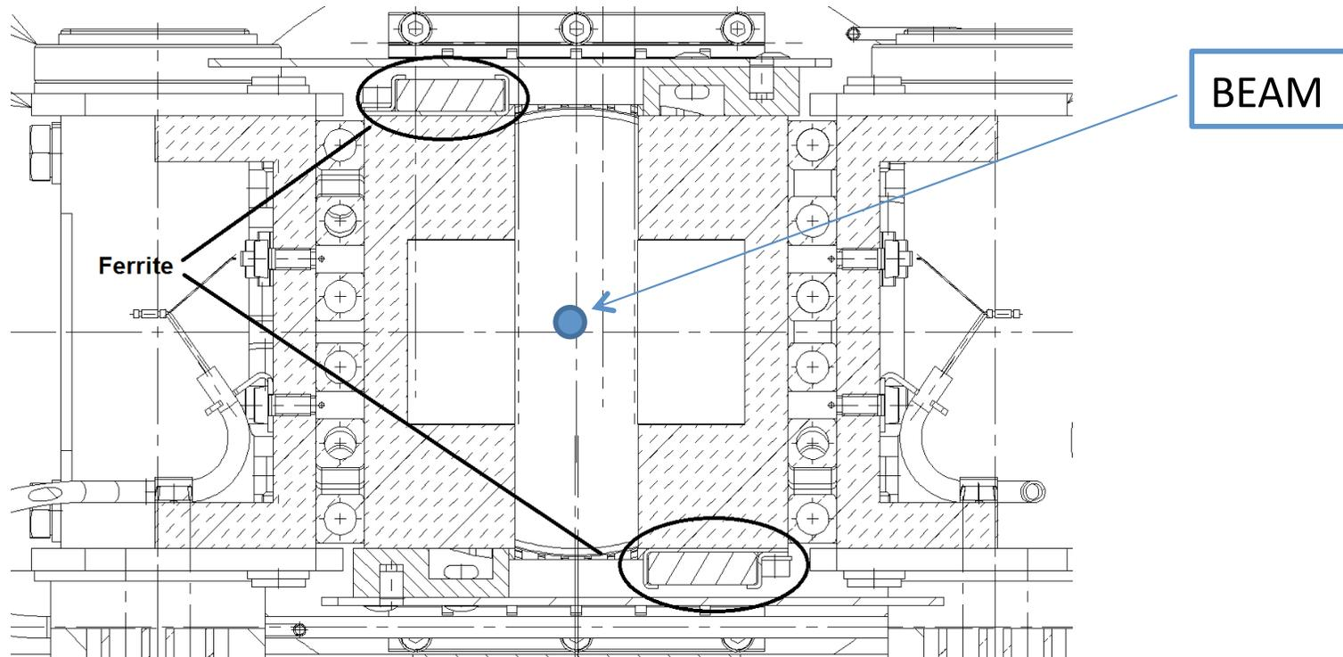
**Total surface of ferrite per collimator = 1600 cm<sup>2</sup>**
