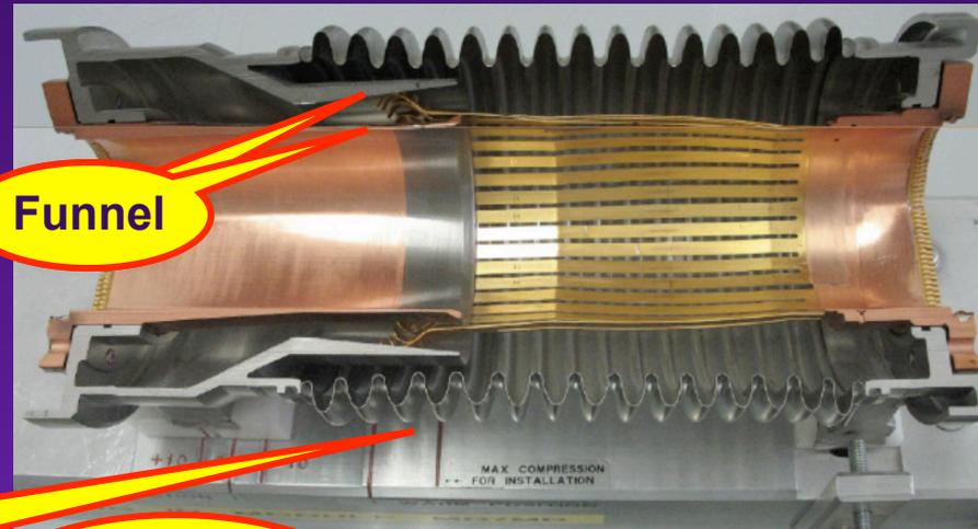
RF contact fingers to shield the distorted geometry of the bellows from the beam
