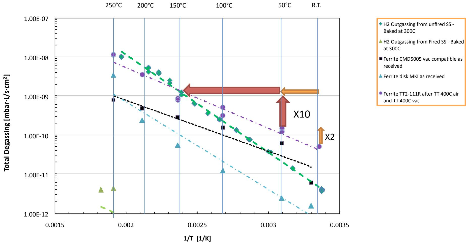
➔ Factor 10 gain in outgassing rate for 100°C temperature increase
