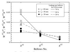
Figure: 6  $W^{\#1}/k^{\#1}$  -  $W^{\#3}/k^{\#1}$  for three slit length,  $l_s = 20$ , 30 and 60 mm.
