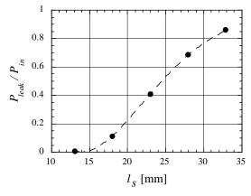
Figure: 4 Change of  $P_{leak}/P_{in}$  against  $l_s$
