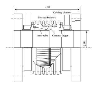
Figure: 1 Schematic drawing of the bellows assembly for the LER of KEKB.
