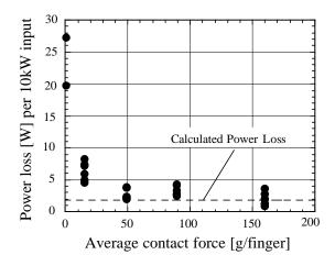
Figure: 3 power loss at the model per 1 kW input for tested contact forces.
