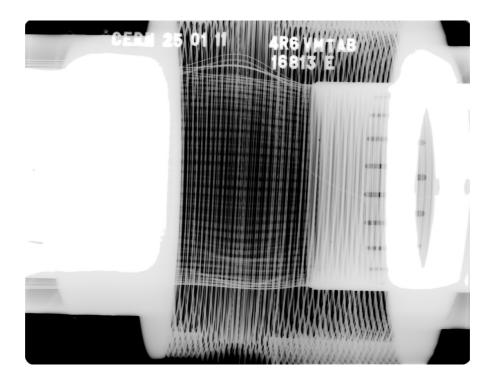
Figure 4 – Image of installed VMTAB bellow in 4R6, showing problem with bulged out contact fingers.
