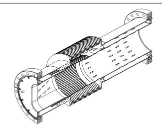
Figure 3 – Section through the VMTAB bellows showing the racetrack to circular transition and RF contact fingers.
