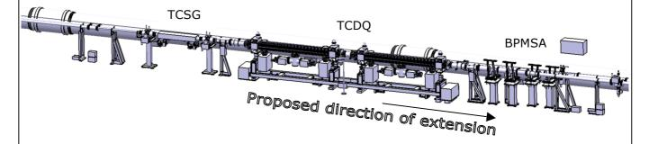
Figure 5 – Integration of the current TCDQ situation in 4L6, showing the possible impact on the BPMSB and TCSG positions. The mirror image applies in 4R6.
