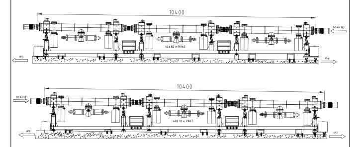
Figure 2 – Proposed layout of the TCDQ system for 4L6.B2 in RA63 (top) and 4R6.B1 in RA67 (bottom).
