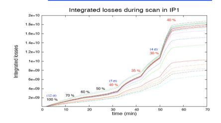
→ Bunch by bunch loss as function of crossing angle in IP1
