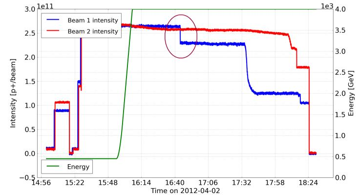
The 1<sup>st</sup> instability in the beam 1 was ~ at 16:43 in the bunch 1, in the horizontal plane
