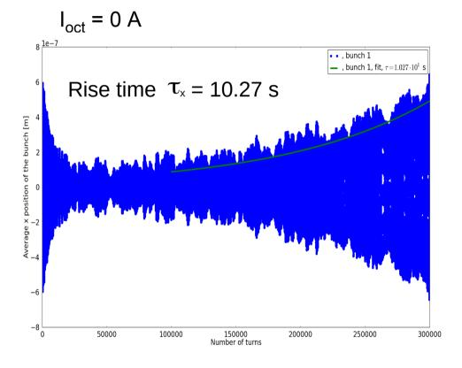
The beam is stable in range of focusing octupole current I =  $-25 \mp 25$  A
