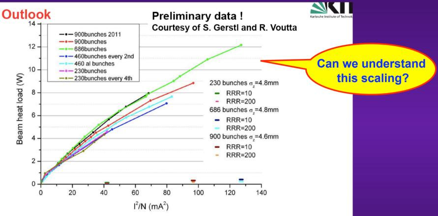
From these preliminary data, we would conclude that the beam heating due to geometrical and resistive wall impedances is not the main mechanism responsible for the beam heat load.
