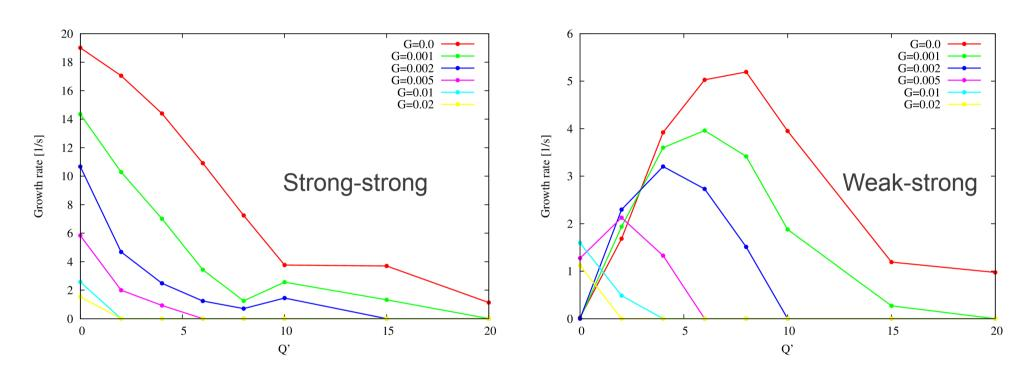
$\rightarrow$  Comparison between strong-strong (tune spread+coherent modes) and weak strong (tune spread only) for the same beam parameters – tune spread ~200A of octupoles
