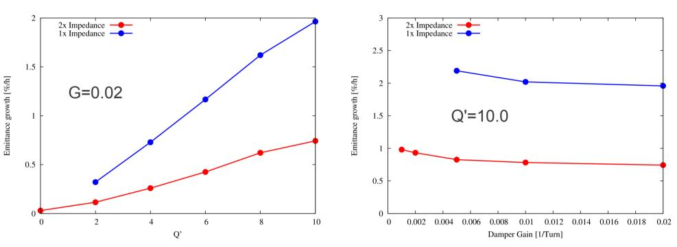
$\rightarrow$  Strong dependency of emittance growth (or lifetime degradation, non losses in the code) with chromaticity – missing points means the beam is unstable
