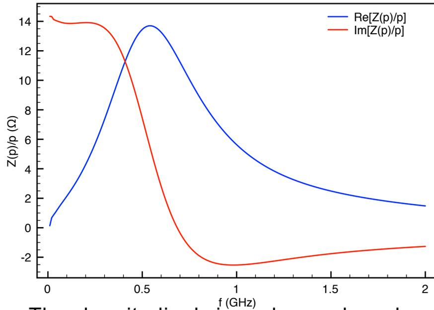
The longitudinal impedance has been evaluated by using the field matching technique (Tsutsui), which was shown to be in good agreement with measurements and CST Microwave Studio simulations
