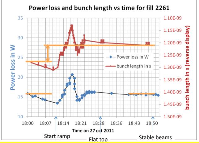
Comparing before and after the ramp  $\rightarrow$  0.05 ns decrease in bunch length seems have no impact on power loss  $\rightarrow$  Not only the bunch length matters but also the distribution (blow up...).
