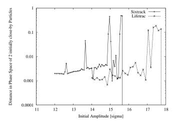
Figure 2: Distance in phase space of two initially close particles after 1E6 turns of tracking vs. the initial amplitude. Beam-beam interaction is off, particles' momentum deviation is 0 (4D case). Initial angle in Ax,Ay plane is 45 degrees.
