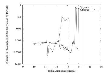
Figure 6: Distance in phase space of two initially close particles after 1E6 turns of tracking vs. the initial amplitude. Beam-beam interaction is off, particles' momentum deviation is 0.00027 (6D case). Initial angle in Ax,Ay plane is 75 degrees.
