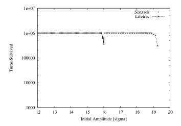
Figure 7: Particle survival time in turns vs. the initial amplitude. Beam-beam interaction is off, particles' momentum deviation is 0 (4D case). Initial angle in Ax,Ay plane is 15 degrees.
