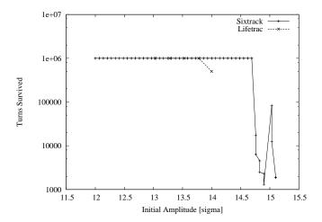
Figure 9: Particle survival time in turns vs. the initial amplitude. Beam-beam interaction is off, particles' momentum deviation is 0 (4D case). Initial angle in Ax,Ay plane is 75 degrees.
