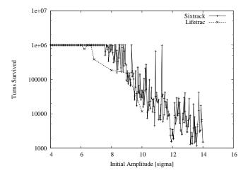
Figure 16: Particle survival time in turns vs. the initial amplitude. Beam-beam interaction is on, particles' momentum deviation is 0 (4D case). Initial angle in Ax, Ay plane is 45 degrees.
