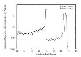
Figure 1: Distance in phase space of two initially close particles after 1E6 turns of tracking vs. the initial amplitude. Beam-beam interaction is off, particles' momentum deviation is 0 (4D case). Initial angle in Ax,Ay plane is 15 degrees.
