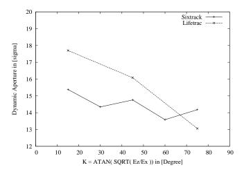
Figure 13: Dynamic aperture in beam sigma vs. initial angle in Ax,Ay plane. Beam-beam interaction is off, particles' momentum deviation is 0.00027 (6D case).
