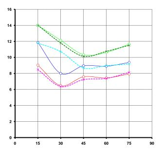
Figure 20: LHC dynamic aperture for the 4D and the 6D BB (13 slices) treatment. The curves in shades of green are DA for 10'000, bluish for 100'000 and reddish for 1'000'000 turns respectively. The solid lines with circles are from the 4D BB while the dashed curves with an "X" character are the results from 6D BB tracking.
