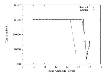
Figure 12: Particle survival time in turns vs. the initial amplitude. Beam-beam interaction is off, particles' momentum deviation is 0.00027 (6D case). Initial angle in Ax,Ay plane is 75 degrees.
