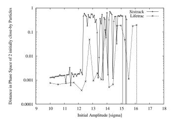
Figure 5: Distance in phase space of two initially close particles after 1E6 turns of tracking vs. the initial amplitude. Beam-beam interaction is off, particles' momentum deviation is 0.00027 (6D case). Initial angle in Ax,Ay plane is 45 degrees.
