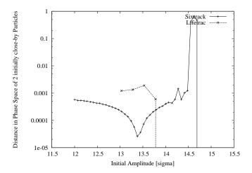
Figure 3: Distance in phase space of two initially close particles after 1E6 turns of tracking vs. the initial amplitude. Beam-beam interaction is off, particles' momentum deviation is 0 (4D case). Initial angle in Ax,Ay plane is 75 degrees.
