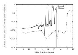
Figure 4: Distance in phase space of two initially close particles after 1E6 turns of tracking vs. the initial amplitude. Beam-beam interaction is off, particles' momentum deviation is 0.00027 (6D case). Initial angle in Ax,Ay plane is 15 degrees.
