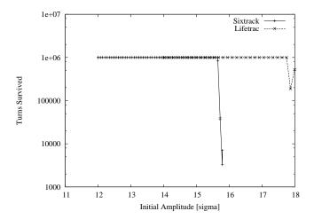
Figure 8: Particle survival time in turns vs. the initial amplitude. Beam-beam interaction is off, particles' momentum deviation is 0 (4D case). Initial angle in Ax,Ay plane is 45 degrees.
