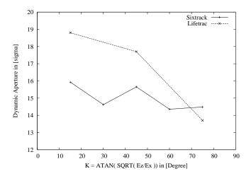
Figure 14: Dynamic aperture in beam sigma vs. initial angle in Ax,Ay plane. Beam-beam interaction is off, particles' momentum deviation is 0 (4D case).
