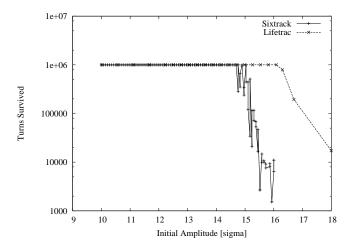
Figure 11: Particle survival time in turns vs. the initial amplitude. Beam-beam interaction is off, particles' momentum deviation is 0.00027 (6D case). Initial angle in Ax,Ay plane is 45 degrees.
