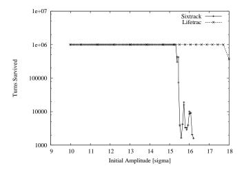
Figure 10: Particle survival time in turns vs. the initial amplitude. Beam-beam interaction is off, particles' momentum deviation is 0.00027 (6D case). Initial angle in Ax,Ay plane is 15 degrees.
