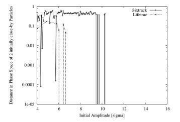
Figure 15: Distance in phase space of two initially close particles after 1E6 turns of tracking vs. the initial amplitude. Beam-beam interaction is on, particles' momentum deviation is 0 (4D case). Initial angle in Ax,Ay plane is 45 degrees.
