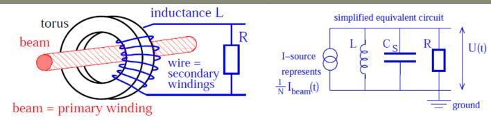
The electrical properties of the transformer and the electronics attached, have to be taken into account to determine the working region where the current measured can be correctly interpreted as a function of the beam current.
