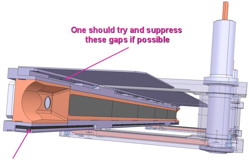
Ferrite (6 mm height but only 3 mm visible by the beam due to the stainless steel box) => Try and increase the visible height of the ferrite
